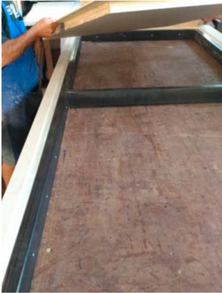
Details of the paneled iron structure and shaped profile of the door before painting.
