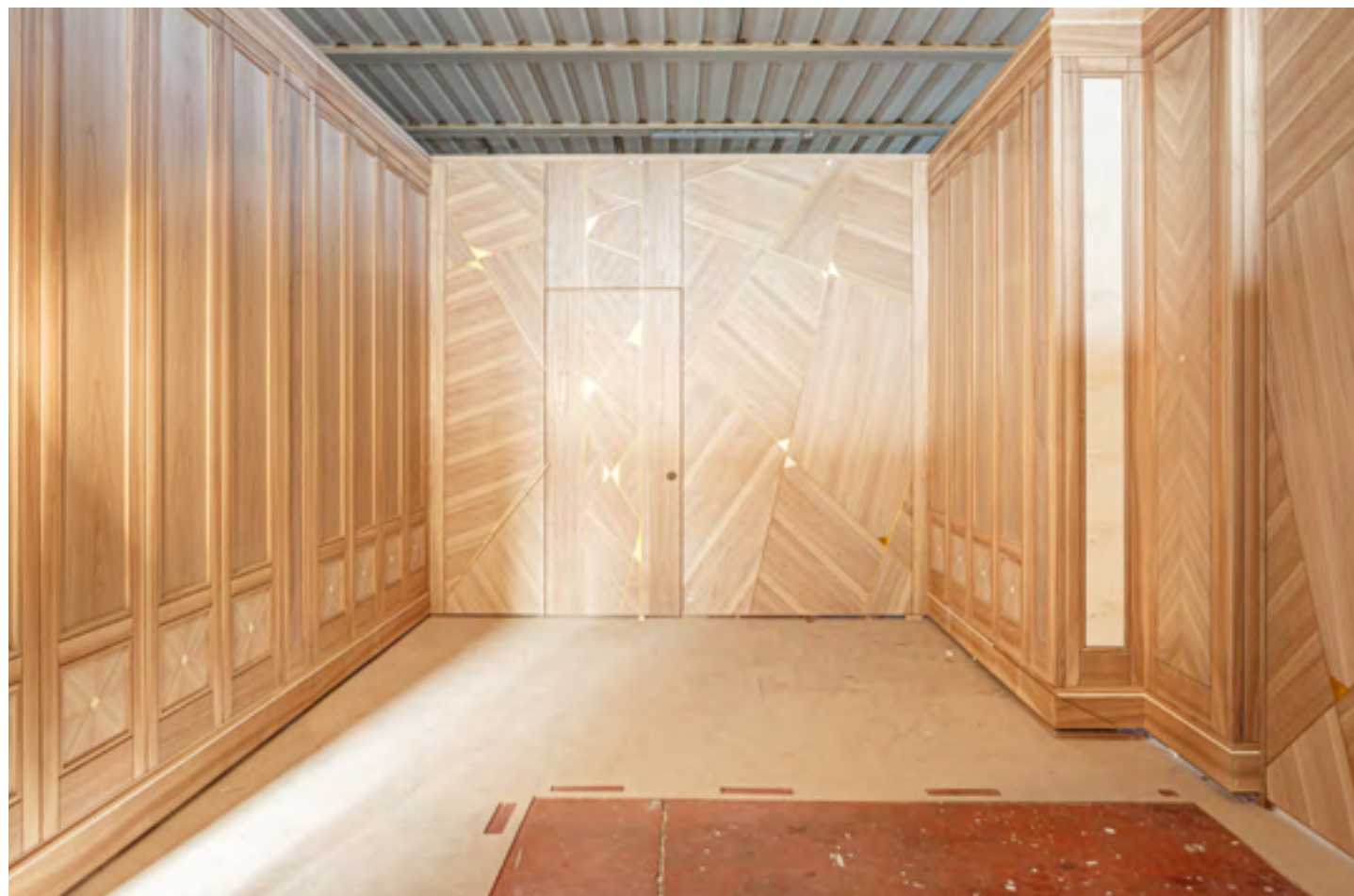
Evocative view of the control and verification of the production of the boiserie by FMF. 1300 square meters of two-tone national walnut selected personally by Franco Martinello.
