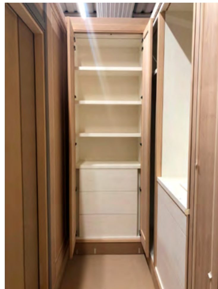
Details in the production phase of the continuous veneer of the plane tree in all the internal elements of the cabin.
